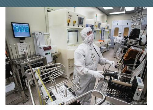
Semiconductor Technicians help manufacture semiconductors with the use of special purpose furnaces, x-ray equipment, chemical baths, and equipment used to form circuitry and change conductive properties.
